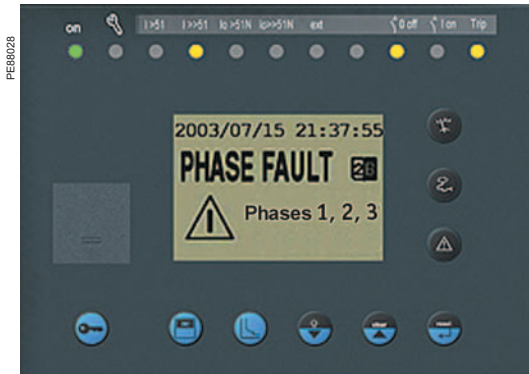
Local indications on the Sepam front panel.
