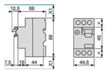
X1: Electrical clearance = 40 mm for Ue < 690 V Mounting
