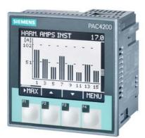
SENTRON, measuring device, 7KM PAC4200, LCD, L-L: 690 V, L-N: 400 V, 5 A, 3-phase, Modbus TCP, optionally Modbus RTU / PROFINET / PROFIBUS / DI/DQ, apparent / active / reactive energy / cos phi, harmonics: 2nd to 64th, THD, Class 0.2 acc. to IEC61557-12 or Class 0.2S acc. to IEC62053-22, wide-range power supply 95 to 240 V +-10% (AC), 110 to 340 V +-10% (DC) screw terminals
