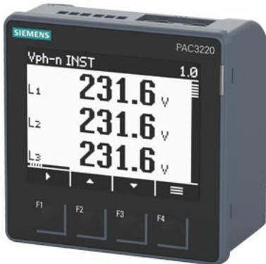
SENTRON PAC3220 LCD 96X96 mm Power Monitoring Device Control panel instrument for electrical values protocol: Modbus TCP with graphics display U rated input: 690/400V 45-65Hz IE rated input: X/1A oder X/5A AC Power supply: 24 ... 60 V -20/+10 % DC screw connections
