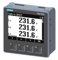
SENTRON PAC1020 96X96 mm Power Monitoring Device Panel mount type for measurement of electr. values Protocol: Modbus RTU With graphical display Un max: 400/230V 45-65Hz Input current 5A AC Power Supply 85V - 276V AC Terminal blocks
