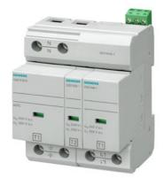
Combination arrester type 1+2 Requirement class B+C, UC 350V Pluggable protective modules 2-pole, 1+1 circuit for TN-S and TT systems with remote display
