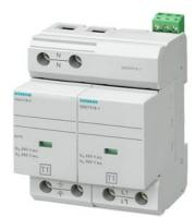
Lightning arresters, type 1 Requirement class B, UC 350V Pluggable protective modules 2-pole, 1+1 circuit for TN-S and TT systems with remote display
