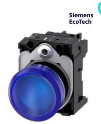
Indicator lights, 22 mm, round, metal, shiny, blue, lens, smooth, with holder, LED module with integrated LED 230 V AC, screw terminal
