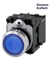
Illuminated pushbutton, 22 mm, round, metal, shiny, blue, pushbutton, flat, momentary contact type, with holder, 1 NO, LED module with integrated LED 24 V AC/DC, screw terminal
