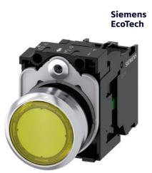
Illuminated pushbutton, 22 mm, round, metal, shiny, yellow, pushbutton, flat, momentary contact type, with holder, 1 NO, LED module with integrated LED 24 V AC/DC, screw terminal
