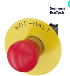
EMERGENCY STOP mushroom-type actuator, 22 mm, round, metal, shiny, red, 40 mm, positive latching, according to EN ISO 13850, pull-to-unlatch mechanism, with yellow backing plate, inscription: NOT-HALT, with holder, 1 NC, screw terminal
