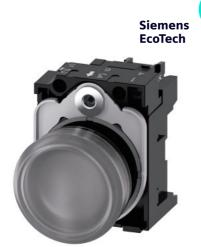
Indicator lights, 22 mm, round, plastic, clear, lens, smooth, with holder, LED module, with integrated LED 24 V AC/DC, screw terminal
