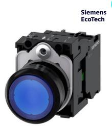
Illuminated pushbutton, 22 mm, round, plastic, blue, pushbutton, flat, momentary contact type, with holder, 1 NO, LED module with integrated LED 24 V AC/DC, screw terminal
