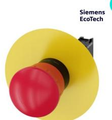
EMERGENCY STOP mushroom pushbutton, 22 mm, round, plastic, red, 40 mm, positive latching, acc. to EN ISO 13850, rotate-to-unlatch, with yellow backing plate, without inscription, with holder, 1 NC, screw terminal
