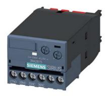
solid-state time-delayed auxiliary switch, off delayed, without control signal, relay 1 NC + 1 NO, time range 0.05-100 s, 24-240 V AC/DC, 50/60 Hz, varistor for attenuation of the contactor coils integrated, screw terminal, can be snapped onto the front on contactors 3RT20 and contactor relays 3RH2
