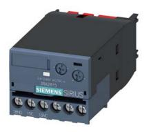
solid-state time-delayed auxiliary switch, off delayed, without control signal, relay: 1 CO, time range 0.05-100 s, 24-240 V AC/DC, 50/60 Hz, varistor for attenuation of the contactor coils integrated, screw terminal, can be snapped onto the front on contactors 3RT20 and contactor relays 3RH2
