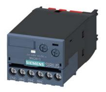
solid-state time-delayed auxiliary switch, ON-delay, relay 1 NC + 1 NO, time range 0.05-100 s, 24-240 V AC/DC, 50/60 Hz, varistor for attenuation of the contactor coils integrated, screw terminal, can be snapped onto the front on contactors 3RT20 and contactor relays 3RH2
