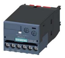
solid-state time-delayed auxiliary switch, ON-delay, relay: 1 CO, time range 0.05-100 s, 24-240 V AC/DC, 50/60 Hz, varistor for attenuation of the contactor coils integrated, screw terminal, can be snapped onto the front on contactors 3RT20 and contactor relays 3RH2
