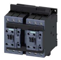
reversing contactor assembly, AC-3e/AC-3, 65 A, 30 kW / 400 V, 3-pole, 230 V AC, 50/60 Hz, screw terminal, electrical and mechanical interlock, auxiliary contacts: 2 x 1 NO
