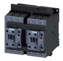
reversing contactor assembly, AC-3e/AC-3, 41 A, 18.5 kW / 400 V, 3-pole, 230 V AC, 50/60 Hz, screw terminal, electrical and mechanical interlock, auxiliary contacts: 2 x 1 NO
