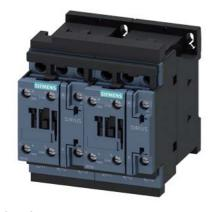
reversing contactor assembly, AC-3e/AC-3, 17 A, 7.5 kW / 400 V, 3-pole, 230 V AC, 50/60 Hz, screw terminal, electrical and mechanical interlock, auxiliary contacts: 2 x 1 NO
