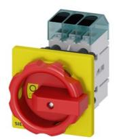
Load disconnector 3LD3, lu 63 A Main switch 3-pole Rated operating capacity at AC-23 A at 400V 22.0 kW Front plate mounting Basic switch with Central hole mounting 22.5mm Toggle drive red / yellow 66x66 mm
