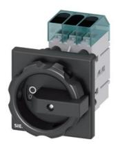
Load disconnector 3LD3, lu 63 A Main switch 3-pole Rated operating capacity at AC-23 A at 400V 22.0 kW Front plate mounting Basic switch with Central hole mounting 22.5mm Toggle drive black 66x66 mm
