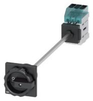
Load disconnector 3LD3, lu 63 A Main switch 3-pole Rated operating capacity at AC-23 A at 400V 22.0 kW floor mounting Basic switch with door coupling Central hole mounting 22.5mm Rotating drive black 66 x 66 mm
