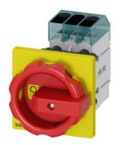
Load disconnector 3LD3, Iu 40 A Main switch 3-pole Rated operating capacity at AC-23 A at 400 V 18.5 kW Front plate mounting Basic switch with Central hole mounting 22.5mm Toggle drive red / yellow 66x66 mm
