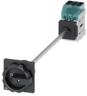
Load disconnector 3LD3, Iu 40 A Main switch 3-pole Rated operating capacity at AC-23 A at 400 V 18.5 kW floor mounting Basic switch with door coupling Central hole mounting 22.5mm Rotating drive black 66 x 66 mm
