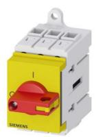
Load disconnector 3LD3, lu 40 A Main switch 3-pole Rated operating capacity at AC-23 A at 400 V 18.5 kW Installation in distribution boards, Basic switch with selector knob red / yellow
