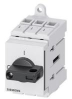
Load disconnector 3LD3, lu 40 A Main switch 3-pole Rated operating capacity at AC-23 A at 400 V 18.5 kW Installation in distribution boards, Basic switch with selector knob black
