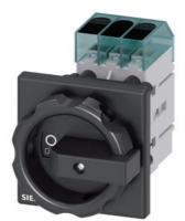
Load disconnector 3LD3, lu 32 A Main switch 3-pole Rated operating capacity for AC-23 A at 400V 11.5kW Front plate mounting Basic switch with Central hole mounting 22.5mm Rotating drive black 66 x 66 mm
