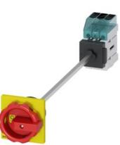
Load disconnector 3LD3, Iu 32 A Main switch 3-pole Rated operating capacity for AC-23 A at 400V 11.5kW floor mounting Basic switch with door coupling Central hole mounting 22.5mm Rotary actuator red / yellow 66 x 66 mm
