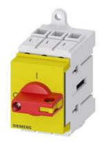
Load disconnector 3LD3, lu 25 A Main switch 3-pole Rated operating capacity at AC-23 A at 400V 9.0kW Installation in distribution boards, Basic switch with selector knob red / yellow
