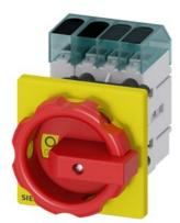
Load disconnector 3LD3, lu 16 A Main switch 3-pole + N Rated operating capacity at AC-23 A at 400V 7.5kW Front plate mounting Basic switch with Central hole mounting 22.5mm Rotary actuator red / yellow 66 x 66 mm
