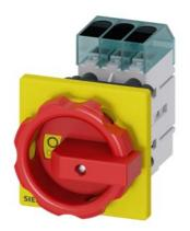
Load disconnector 3LD3, Iu 16 A Main switch 3-pole Rated operating capacity at AC-23 A at 400V 7.5kW Front plate mounting Basic switch with Central hole mounting 22.5mm Rotary actuator red / yellow 66 x 66 mm
