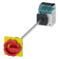
Load disconnector 3LD3, Iu 16 A Main switch 3-pole + N Rated operating capacity at AC-23 A at 400V 7.5kW floor mounting Basic switch with door coupling Central hole mounting 22.5mm Rotary actuator red / yellow 66 x 66 mm
