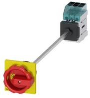
Load disconnector 3LD3, lu 16 A Main switch 3-pole Rated operating capacity at AC-23 A at 400V 7.5kW floor mounting Basic switch with door coupling Central hole mounting 22.5mm Rotary actuator red / yellow 66 x 66 mm
