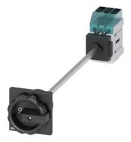
Load disconnector 3LD3, Iu 16 A Main switch 3-pole Rated operating capacity at AC-23 A at 400V 7.5kW floor mounting Basic switch with door coupling Central hole mounting 22.5mm Rotating drive black 66 x 66 mm
