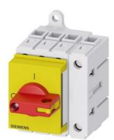
Load disconnector 3LD3, Iu 16 A Main switch 3-pole + N Rated operating capacity at AC-23 A at 400V 7.5kW Installation in distribution boards, Basic switch with selector knob red / yellow
