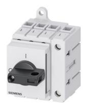
Load disconnector 3LD3, Iu 16 A Main switch 3-pole + N Rated operating capacity at AC-23 A at 400V 7.5kW Installation in distribution boards, Basic switch with selector knob black
