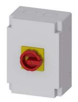
SENTRON, Switch disconnector 3LD, emergency switching-off switch, 3- pole, lu: 125 A, operating power / at AC-23 A 400 V: 45 kW, Molded plastic encapsulation for metric cable gland, rotary operating mechanism, red/yellow
