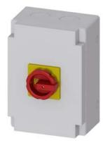
SENTRON, Switch disconnector 3LD, emergency switching-off switch, 3- pole, lu: 100 A, operating power / at AC-23 A 400 V: 37 kW, Molded plastic encapsulation for metric cable gland, rotary operating mechanism, red/yellow
