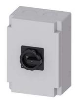
SENTRON, Switch disconnector 3LD, main switch, 3-pole, lu: 100 A, Operating power / at AC-23 A at 400 V: 37 kW, molded-plastic encapsulation for metric cable gland, rotary operating mechanism, black
