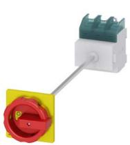
SENTRON, Switch disconnector 3LD, emergency switching-off switch, 3- pole, lu: 100 A, operating power / at AC-23 A 400 V: 37 kW, floor mounting with door coupling, rotary operating mechanism, Red / yellow, 4-hole mounting of the handle
