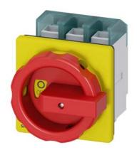
SENTRON, Switch disconnector 3LD, emergency switching-off switch, 3- pole, lu: 100 A, operating power / at AC-23 A 400 V: 37 kW, front-mounted, rotary operating mechanism, Red / yellow, 4-hole mounting of the handle
