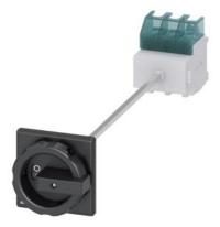
SENTRON, Switch disconnector 3LD, main switch, 3-pole, lu: 63 A, Operating power / at AC-23 A at 400 V: 22 kW, floor mounting with door coupling, rotary operating mechanism, black, 4-hole mounting of the handle
