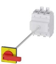
SENTRON, Switch disconnector 3LD, emergency switching-off switch, 3- pole, lu: 160 A, operating power / at AC-23 A 400 V: 75 kW, floor mounting with door coupling, knob-operated mechanism, red/yellow, 4-hole mounting of the handle
