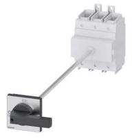
SENTRON, switch disconnector 3LD, main switch, 3-pole, lu: 160 A, operating performance / at AC-23 A at 400 V: 75 kW, floor mounting with door coupling, knob-operated mechanism, black, 4-hole mounting of the handle,
