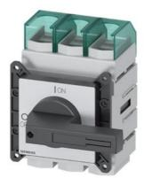
SENTRON, Switch disconnector 3LD, main switch, 3-pole, lu: 160 A, Operating power / at AC-23 A at 400 V: 75 kW, front-mounted, knob-operated mechanism, black, 4-hole mounting of the handle
