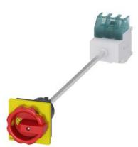
SENTRON, Switch disconnector 3LD, emergency switching-off switch, 3- pole, lu: 32 A, operating power / at AC-23 A 400 V: 11.5 kW, floor mounting with door coupling, rotary operating mechanism, Red / yellow, 4-hole mounting of the handle
