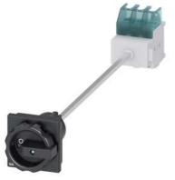
SENTRON, Switch disconnector 3LD, main switch, 3-pole, Iu: 32 A, Operating power / at AC-23 A at 400 V: 11.5 kW, floor mounting with door coupling, rotary operating mechanism, black, 4-hole mounting of the handle
