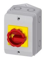
SENTRON, Switch disconnector 3LD, emergency switching-off switch, 3- pole, lu: 25 A, operating power / at AC-23 A 400 V: 9.5 kW, Molded plastic encapsulation for metric cable gland, rotary operating mechanism, red/yellow
